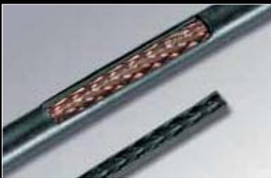
Removing cable insulation
